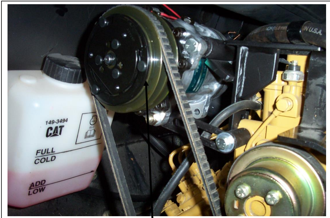
Compressor mounted in place with tightener bracket and belt.
