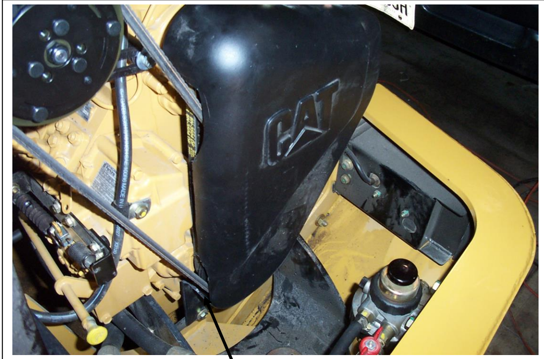
Belt guard with cut outs for new compressor belt.
